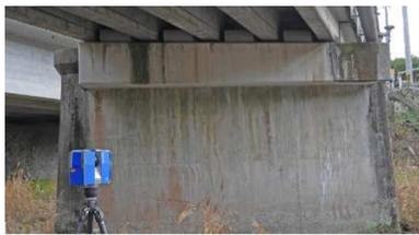
Fig. 6 3D laser scanning
