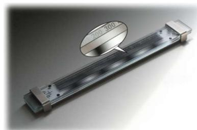
Fig. 1 Schematic illustration of the strain visualization device (SVD)
