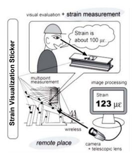
Figure 1. Concept of a proposed Strain Visualization Sticker
