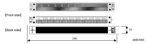
Figure 6. The Developed Strain Visualization Sticker
