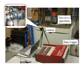
Figure 8. Apparatus for compression test
