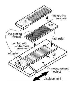
Figure 3. Construct of Strain Visualization Sticker
