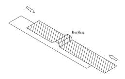
Figure 12. Schematic diagram of film buckling phenomenon
