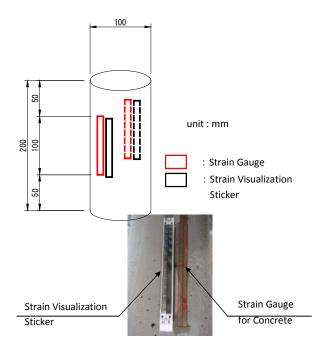
Figure 7. Specimen for compression test
