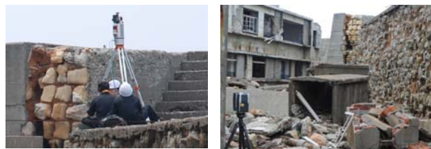
Fig. 3 The situation of measuring using 3D laser scanner
