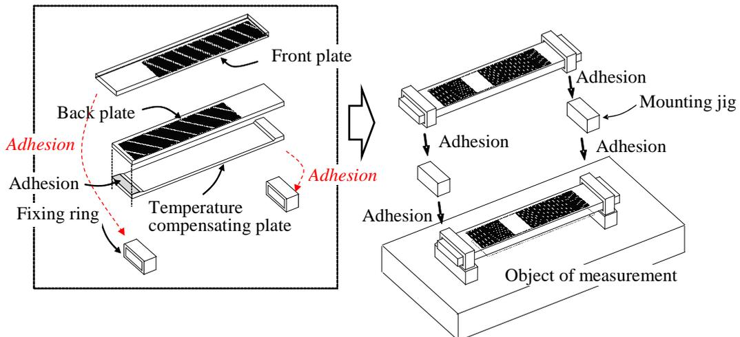
Fig.7 Structure of Strain Visualization Sheet
