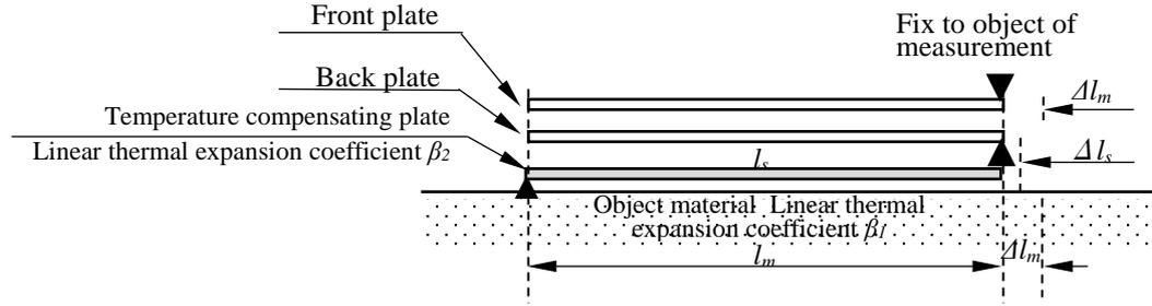
Fig. 5 Proposed self-temperature compensated structure
