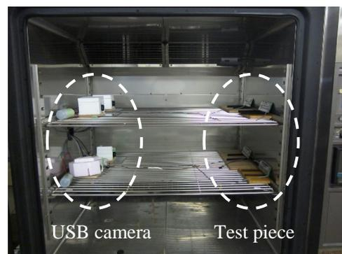
Fig.10 Installation of test piece and USB camera in the thermostatic chamber
