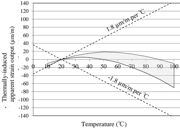
Fig.1 Typical characteristic curve of thermally-induced apparent strain with strain gauges
