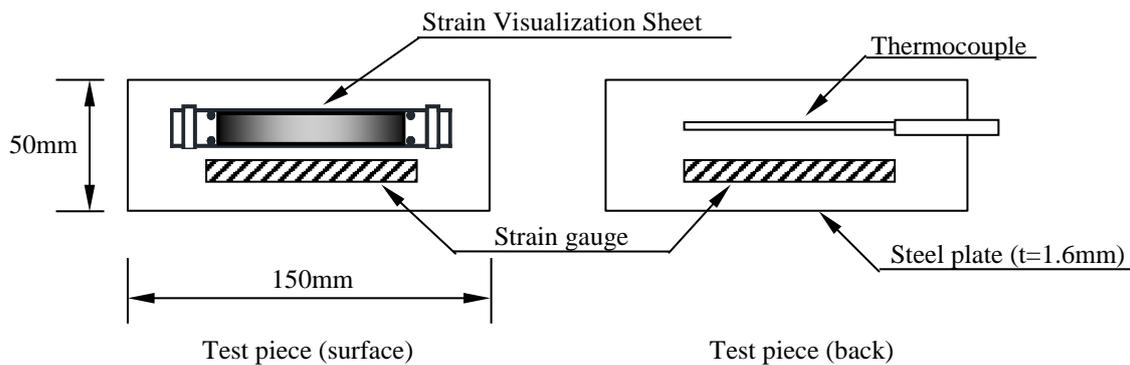
Fig.8 Sensor arrangement
