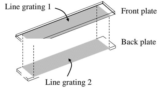
Fig.2 Basic Structure of Strain Visualization Sheet
