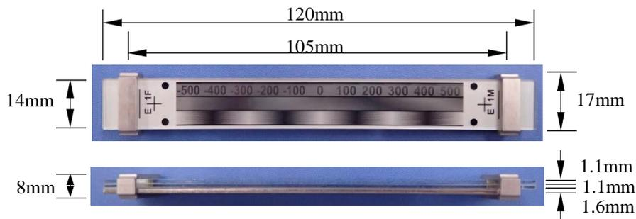
Fig. 6 Appearance of Strain Visualization Sheet
