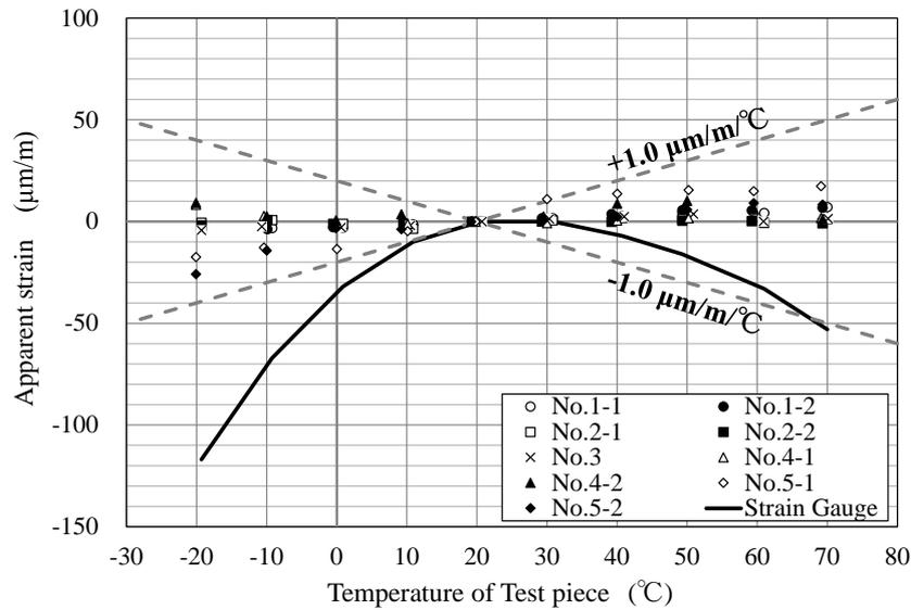
Fig. 11 Relationship between temperature and apparent strain of test piece
