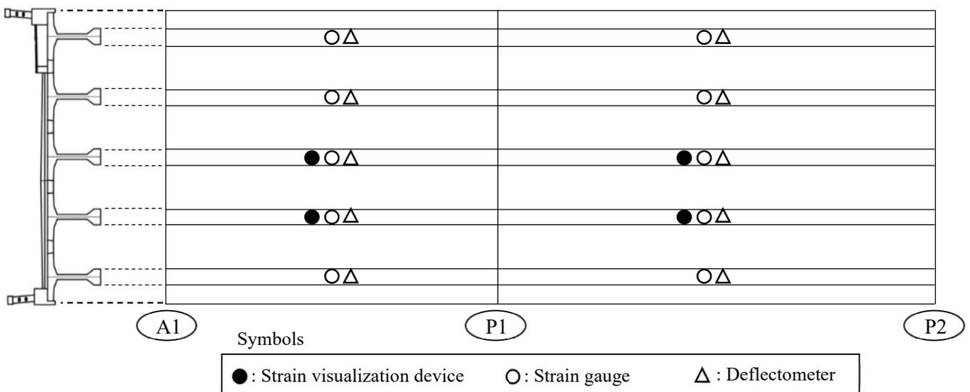
Figure 9. Arrangement of measuring devices
