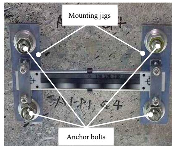
Figure 10. Condition of installation of a strain visualization device
