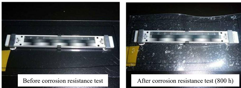
Figure 5. Condition of strain visualization device before (left) and after (right) the corrosion resistance performance test
