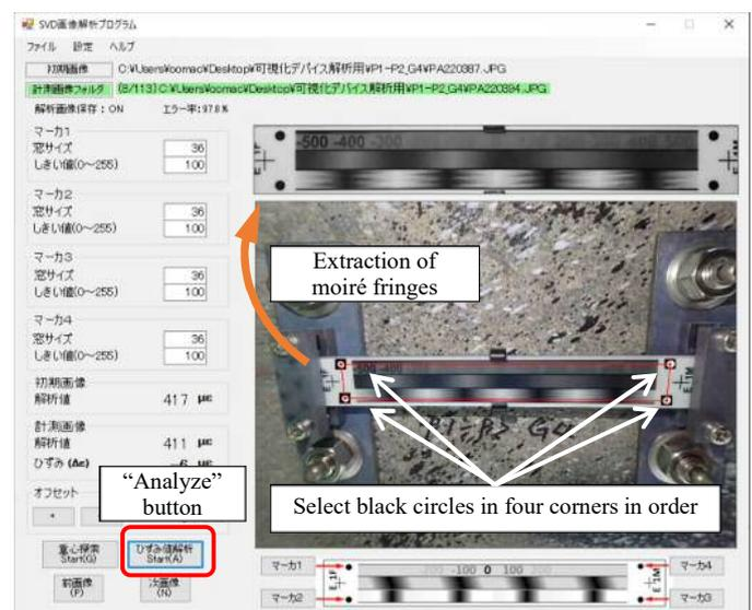
Figure 7. Strain calculation application
