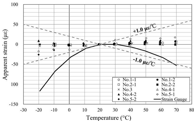
Figure 4. Relationship of specimen temperature and apparent strain
