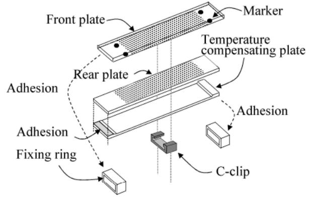
Figure 3. Structure of Strain Visualization Device
